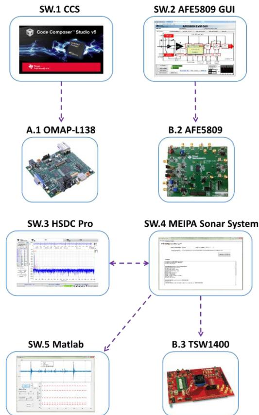
**Figure 13:** Software Block Diagram
