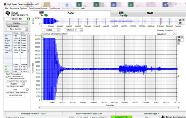
**Figure 19:** Received echo shown in PC by HSDC Pro software
