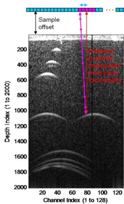
Figure 2: Geometry of Propagation Paths[1]
