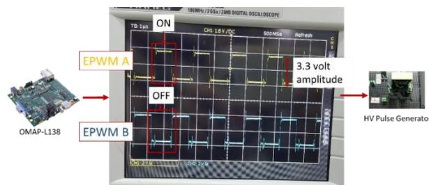
**Figure 6:** two ePWM signals generated by OMAP-L138 with 95Khz frequency and 3.3 volt amplitude
