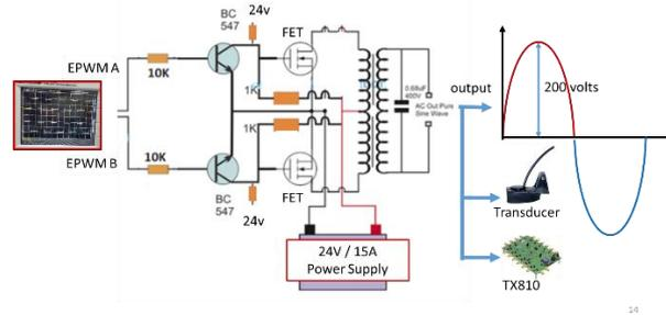
**Figure 8:** Schematic of HV Pulse Generator
