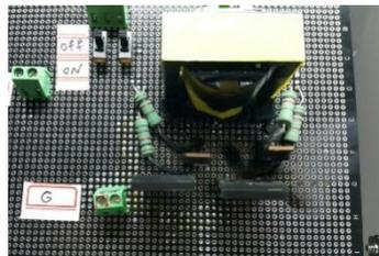
**Figure 7:** HV Pulse Generator Board
