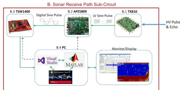
**Figure 9:** Receive Path Sub-Circuit
