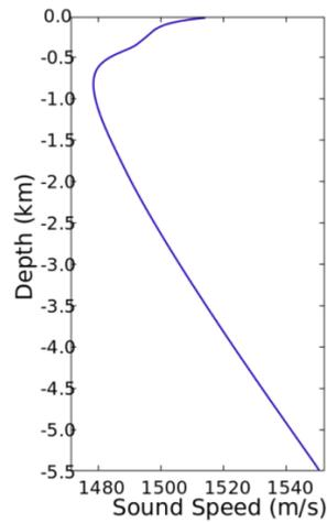
**Figure 3:** Speed of Sound Profile in Sea Water [10]
