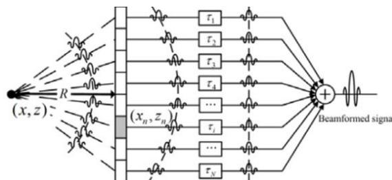
Figure 1: Principle of Delay-and-Sum Beamforming[1]
