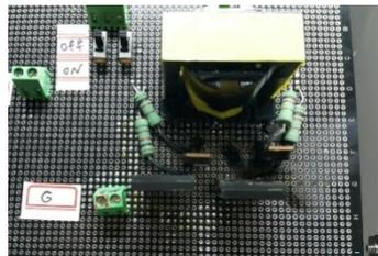
**Figure 7:** HV Pulse Generator Board
