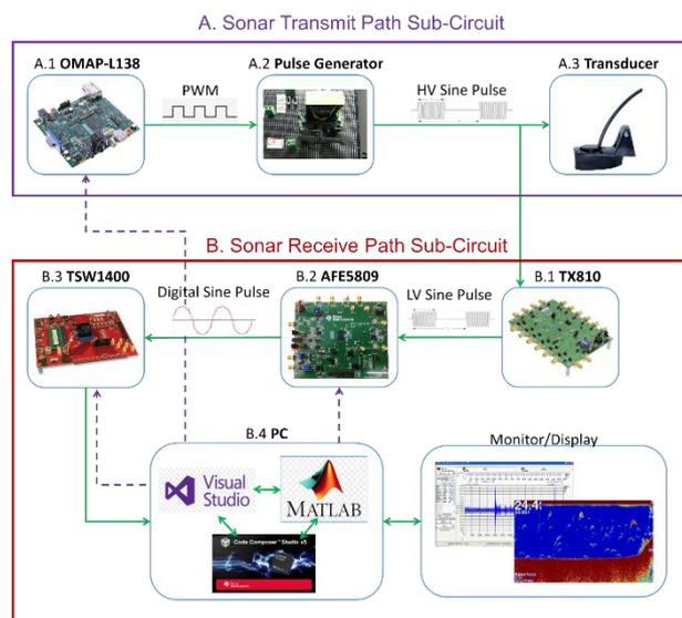
**Figure 4:** Sonar System Diagram
