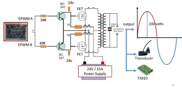
**Figure 8:** Schematic of HV Pulse Generator
