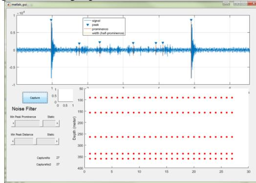
**Figure 14:** Fish Finder GUI, Transmitted pulse and received echo
