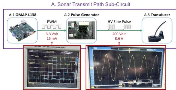
**Figure 5:** Sonar Transmit Path Sub-Circuit
