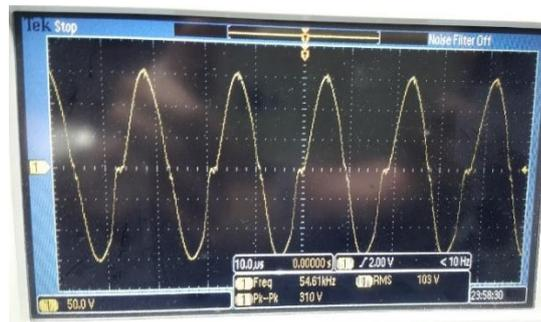
**Figure 16:** HV Pulse Generator output after (Pulse Zoomed-In) after transforming the square shape into sine shape
