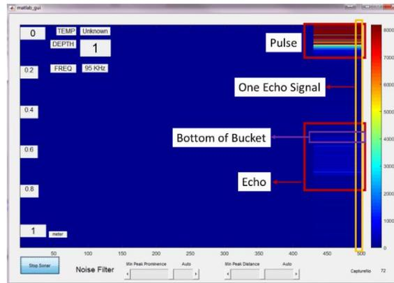
**Figure 20:** Fish Finder GUI: Showing signal results in colorjet
