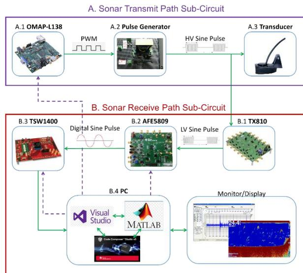
**Figure 4:** Sonar System Diagram
