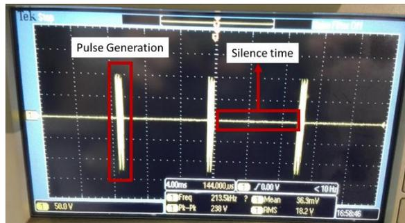
**Figure 17:** Final HV pulse generator output (pulse package)
